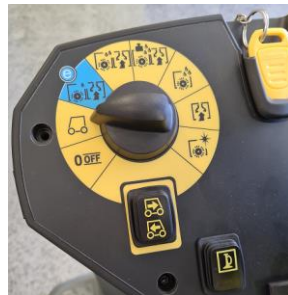
Step 16 Turn the program selector to transport mode
