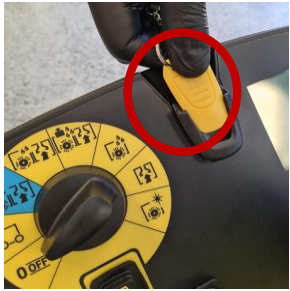
Step 7 Insert the yellow operator KIK key
