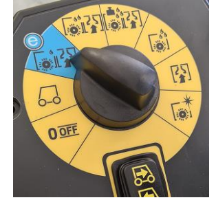
Step 13 Select the relevant cleaning mode. The brush/pad head and squeegee will lower automatically when the drive pedal is pressed
