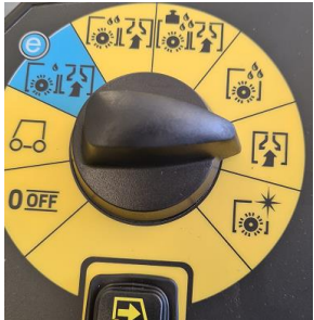
Step 14 When floor scrubbing is finished, set the program selection switch to suction/vacuum
