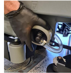
Step 25 Slowly unscrew the filter cap of the fresh water filter and let the fresh water tank drain completely. Replace the filter cap and ensure no water leaks
