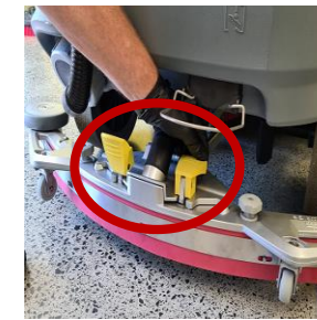
Step 26 Kneel with kneeling pad, lift the yellow handles to release squeegee. Use 2 hands and keep your back straight to lower to the ground, before using SMART moves to lift and move over the drain area
