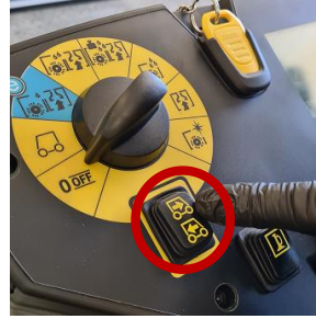
Step 9 Set the drive direction with the drive direction button ➔ Forward ➔ Reverse
