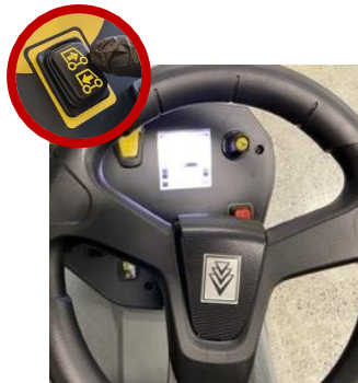
Step 15 Briefly drive forward for approx. 10 metres to suck up the remaining water
