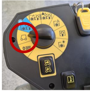
Step 8 Turn the program selector switch to position 1 "Transport mode"
