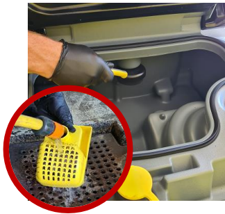
Step 21 Rinse the waste water tank and debris basket
