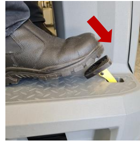
Step 10 Determine the driving speed by pressing the pedal
