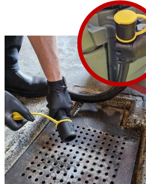
Step 19 Take the water discharge hose from the support and lower above a suitable drain. Twist slowly to open
