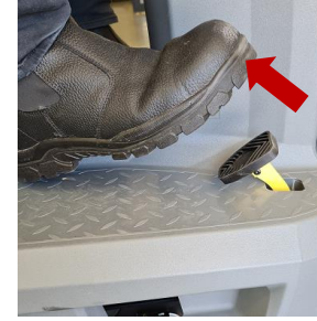
Step 11 To stop, release the drive pedal
