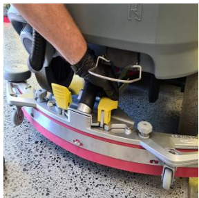
Step 28 Return squeegee to the machine. Use SMART moves to lower it to the ground, kneel with a kneeling pad, use 2 hands, keep your back straight lift it into place
