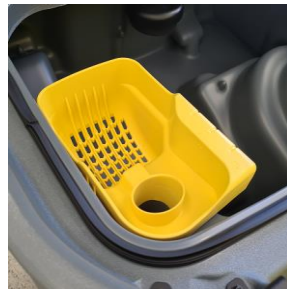
Step 22 Place basket back into the waste water tank
