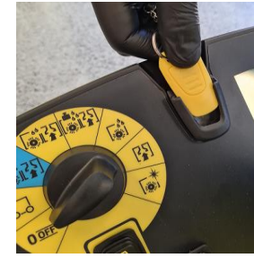
Step 32 Move machine to the correct storage area, remove the KIK key
