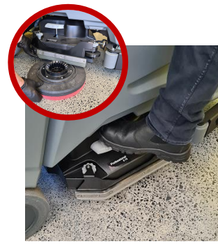
Step 30 Remove pads by pushing the pedal
