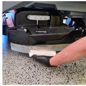
Step 29 Wipe skirt clean with a damp cloth
