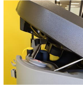
Step 24 Leave the cover open to allow it to dry
