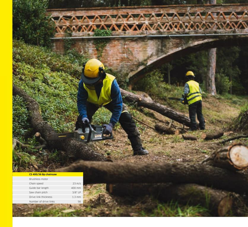
A chainsaw places requirements on battery technology like no other tool. Here our 36 V batteries deliver full power to the chain.
