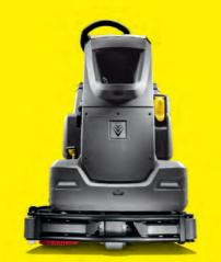
The **B 110 R ride-on scrubber dryer** makes cleaning large areas, such as in supermarkets, airports and warehouses, even more convenient and efficient. The newly developed ride-on machine is ergonomically designed and delivers the best cleaning results with increased productivity. A further highlight: the water supply adjusts to the speed, which significantly reduces water consumption. The machine is also extremely durable and quiet on the move.
