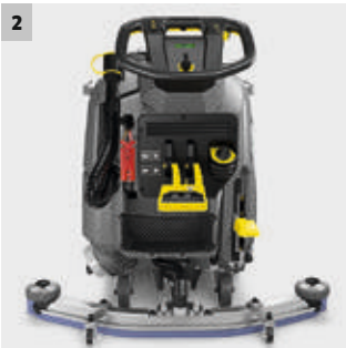
1 The brush head and squeegee are made from long-lasting aluminium
