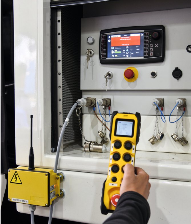
Connected transceiver at the control cabinet
