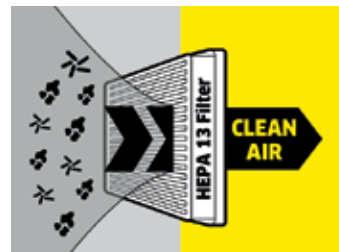
HEPA 13 Filter - Filters 99.95% of all particles larger than 0.3µm
