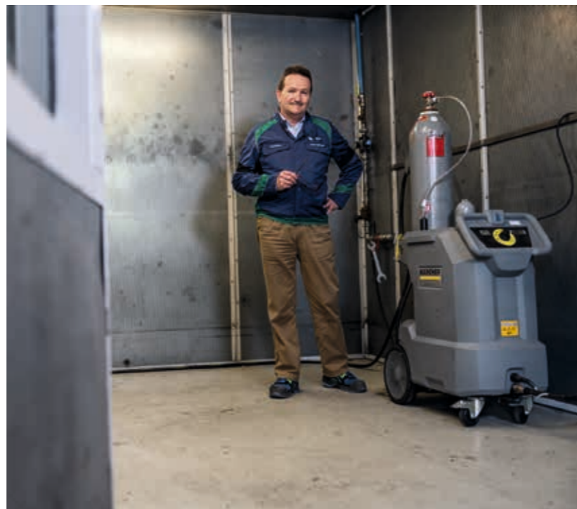
The L2P machine produces dry ice from CO 2 during cleaning. That impressed Alfred Weber and his team.
