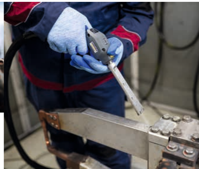
Before maintenance is carried out, the tools are cleaned with dry ice gently, quickly and on site.
