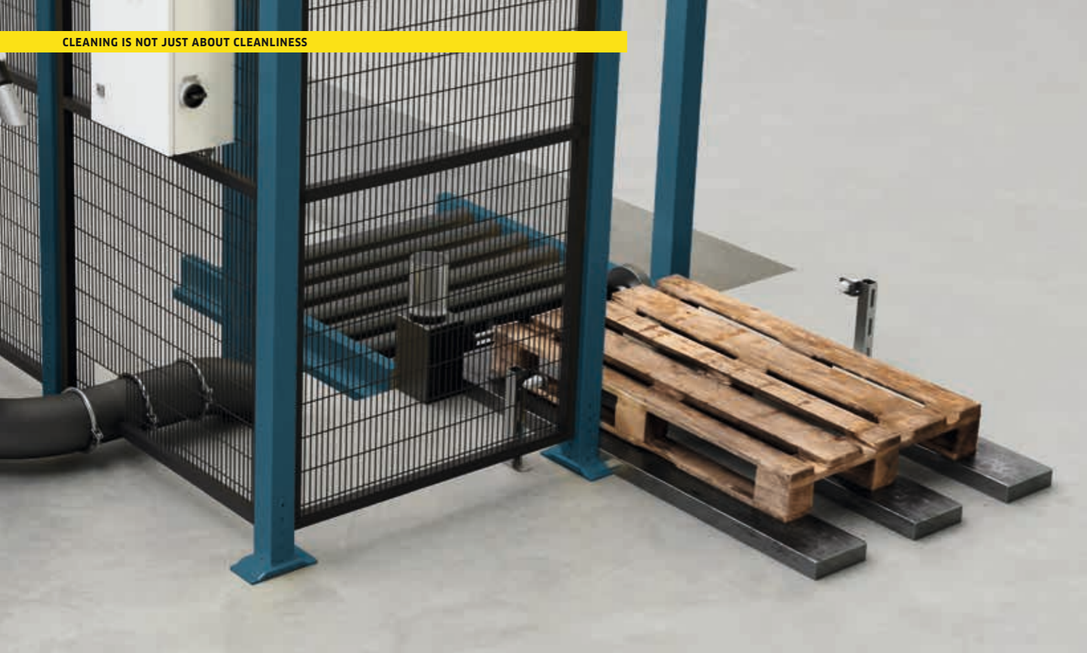
The pallet is guided into the warehouse via a feed-in system.
