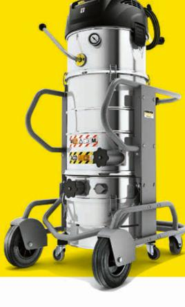
IVM 60/24-2 M ACD WS The specialist for inerting dust at risk of self ignition and explosion such as aluminium, titanium and magnesium, which arises during grinding, pre-separator has an impressive air flow\* of around 530 m<sup>3</sup>/h as well as compact dimensions. The suction material is wetted in the liquid bath and the solid substances are separated in the filter fleece.
