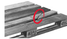
A board is broken transversally or diagonally.
