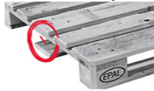
A block is missing or split in such a way that more than one nail shank is visible. Twisted blocks must not protrude more than 10 mm.
