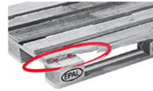
Twisted blocks must not protrude more than 10 mm.
