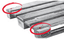
A bottom or deck board is splintered in such a way that more than one nail shank is visible.
