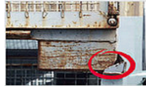
The base frame or feet are bent in such a way that the box pallet no longer stands evenly on four feet or can no longer be safely stacked.
