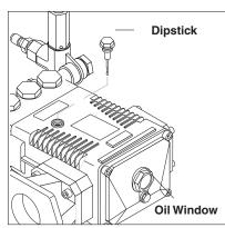
STEP 2: Remove shipping cap and install oil dipstick. Check pump oil level by using dipstick or observe oil level in oil window (if equipped). Use 40 wt. non detergent oil. The Lagacy Axial Pump does not require maintenance. Attemping to check oil on this pump may damage it and will void your pump warranty.
