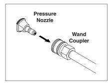
**STEP 6:** Pull spring-loaded collar of the wand coupler back to insert your choice of pressure nozzle.
