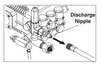
STEP 6: Disconnect the high pressure hose from discharge nipple.
