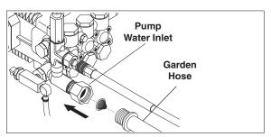
**STEP 10:** Check inlets filters, remove debris, then connect the garden hose to pump water inlet. *CAUTION: Do not run the pump without water or pump damage will result.*
