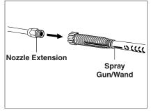
**STEP 5:** Attach nozzle extension to spray gun/wand. Tighten both by hand.
