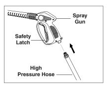
**STEP 4:** Attach the high pressure hose to the spray gun using teflon tape on hose threads.
