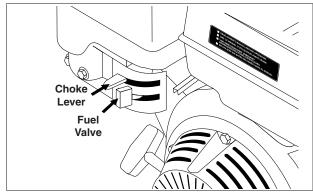
**STEP 7:** Move the choke lever to the "Choke" position (on a warm engine, leave the choke lever in the run position). Move the choke lever to the "Closed" position. To restart a warm engine, leave the choke lever in the "Open" position.
