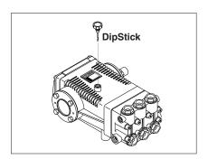
**STEP 7:** Remove shipping cap and install oil dipstick. Check pump oil level by using dipstick or observe oil level in oil window (if equipped). Use 40 wt. (non detergent) oil.
