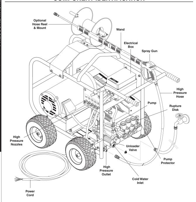
**Pump** — Delivers a specific gpm to the high pressure nozzle which develops pressure.
