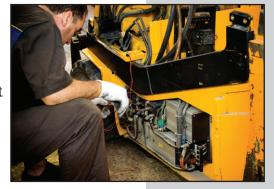
undercarriages and wheel wells of equipment that come under constant attack from dirt and debris. An inspection is only as good as the ability to see problems by the person doing the inspecting. There is more to be seen when you keep it clean.
