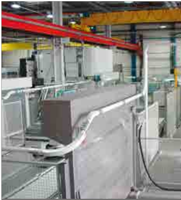
● Suction point with swivel arm and pipeline
