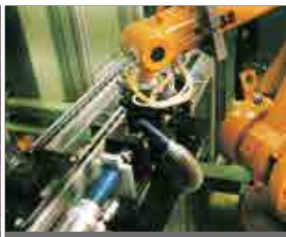
Ringler Kärcher Group suction nozzle for precise vacuuming of milling chips
