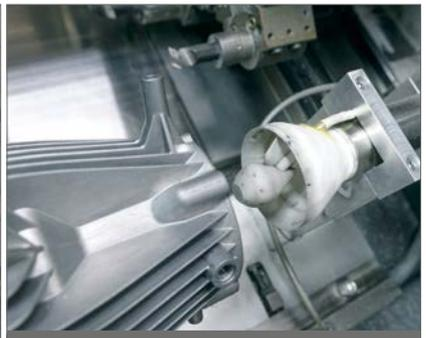
3D-printed nozzle for special vacuum functions
