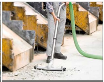
Vacuuming mineral residues, for example concrete
