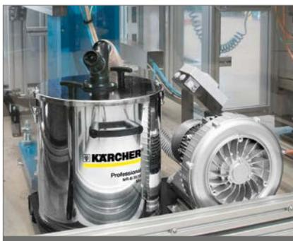
IVR-B 30/15 Me integrated into robot cell
