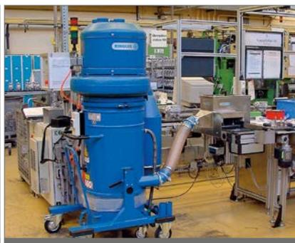
Integrated dust remover in production lines
