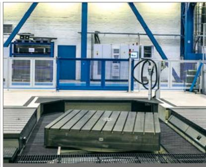
Rolled out vacuuming point for large-scale machining areas
