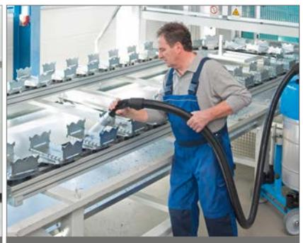
Swarf and coolant vacuuming for machine and plant maintenance and for cleaning of working pieces
