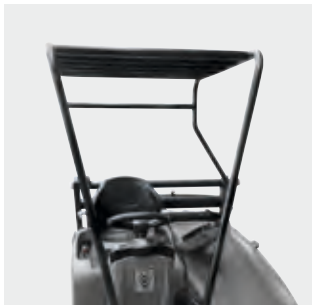
Protective roof Protective roof is compulsory in high-bay warehouses. For reliable and effective protection.
