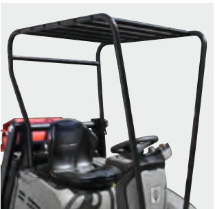
Protective roof Protective roof is compulsory in high-bay warehouses. For reliable and effective protection.
