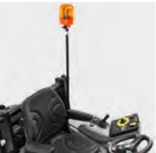
Flashing beacon For attaching to the machine itself or on the protective roof. Improved safety for the user and those in the vicinity.
