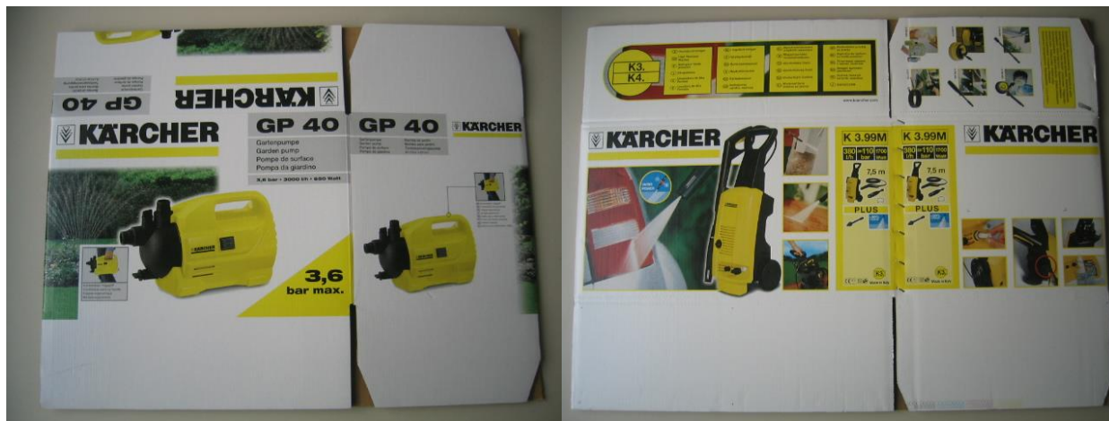
Box on left with glue lap and box on right with staple lap.
