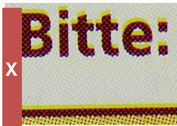
Figure 6: Inaccurate registration, here during offset (yellow exhibits large variation). [9] May result in blurry print results when all colours vary slightly.
