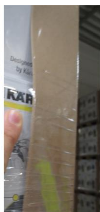
Edge guard taped to package. Reason: interlocked stacking.
