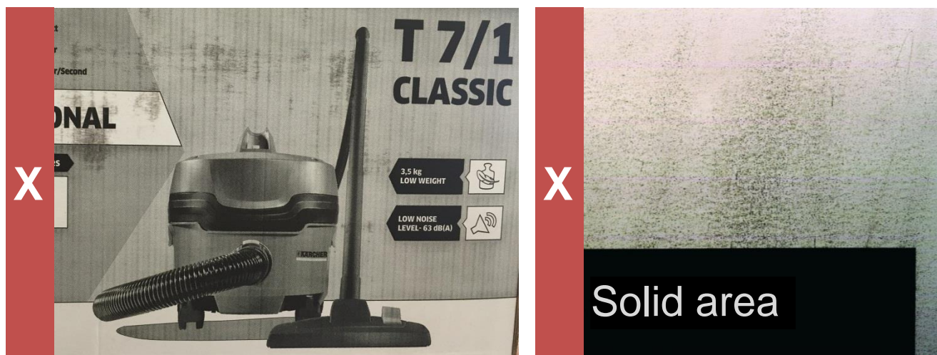
Figure 4: Washboard effect in post-printing and smearing. Right [7] Smearing or chalking after ink is dry due to inadequate smudge resistance. May result in blurry print results.
