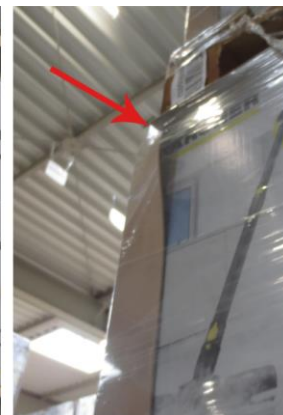
Edge guard bearing load. Result: compressed.
