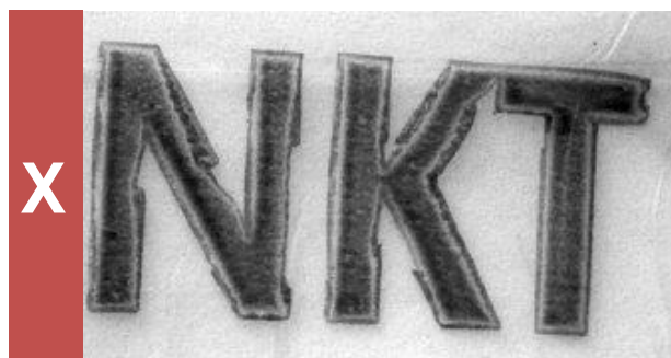
Figure 5: Overly squeezed edges caused by flexo printing. [8]
