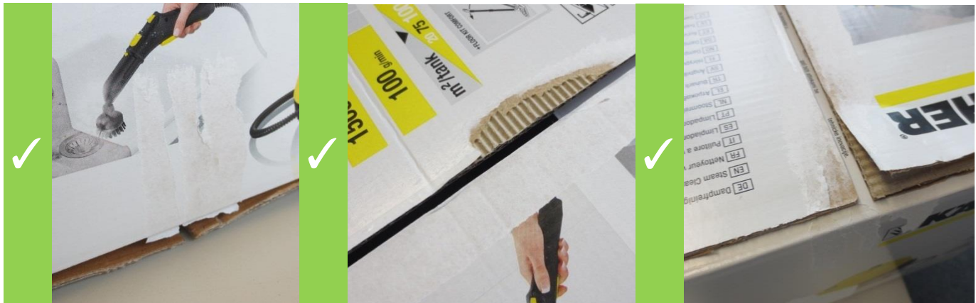
Examples of good tape peeling results (tape takes some of the fibre material with it)
