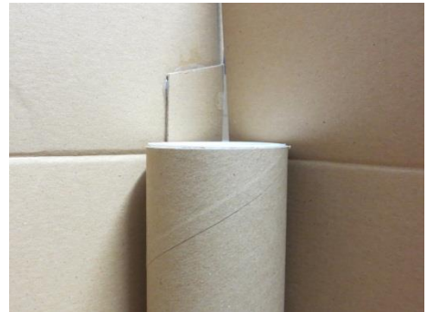
Protruding cardboard tube in packaging undergoing testing.
