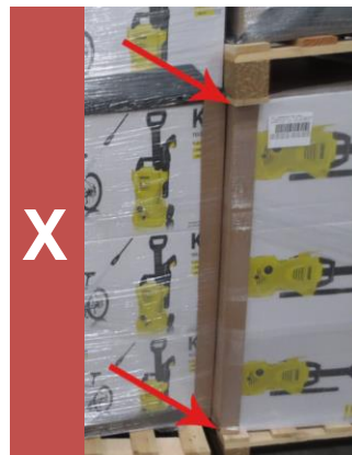
Edge guard bearing load. Result: compressed.
