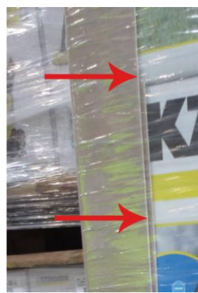
Edge guard bearing load. Result: compressed.
