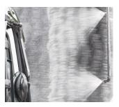
**Perfect cleaning results** An effective chemical pre-spray system cleans with a high-pressure pump with up to 60 bar pressure.
